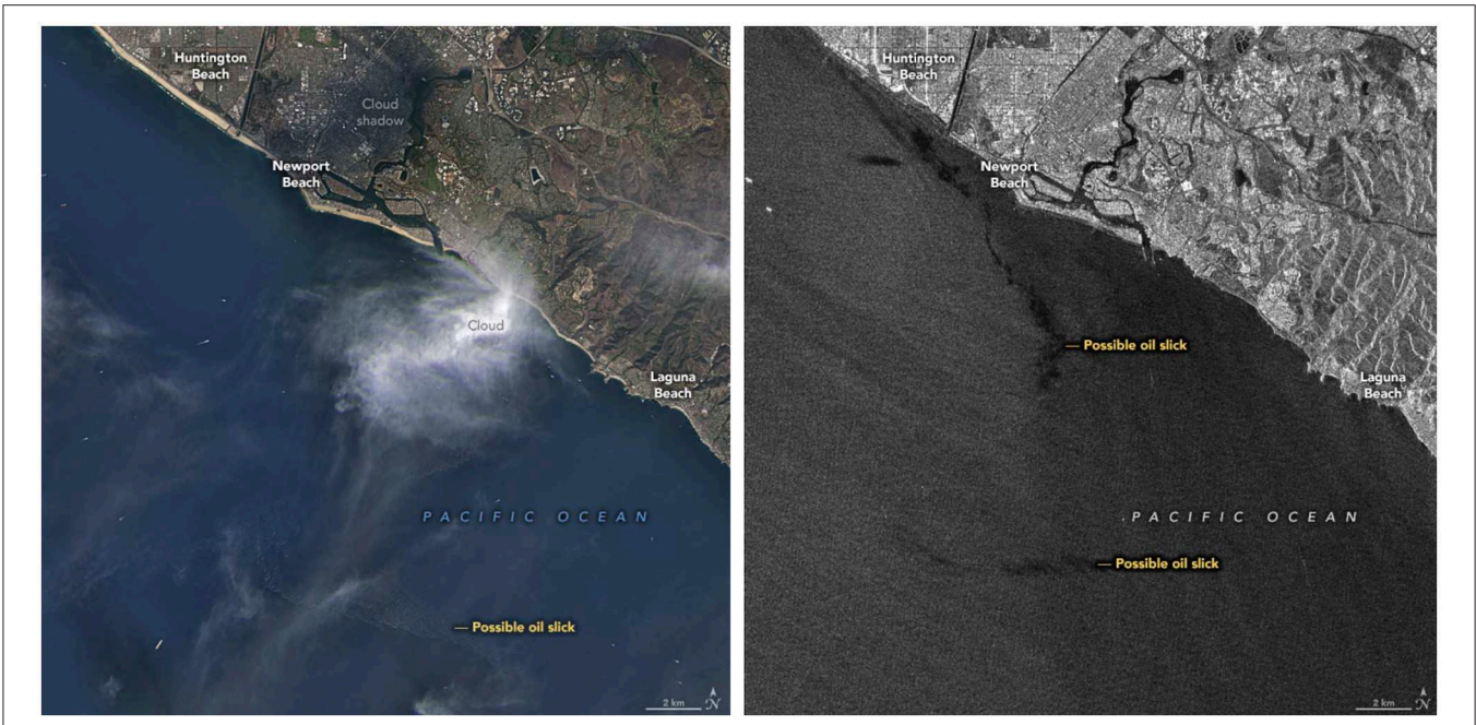
FIGURE 6 | Satellites were able to spot an oil slick from a major oil spill in Southern California in 2021. (L) is an image from October 2, 2021, from OLI on Landsat 8, and (R) is a SAR image from the ESA Sentinel-1B satellite. [Credit: NASA Earth Observatory image by Joshua Stevens, using Landsat data from the U.S. Geological Survey and modified Copernicus Sentinel data processed by the ESA (NASA Earth Observatory, 2021b)].
