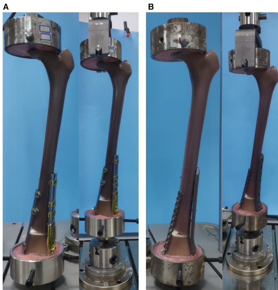
FIGURE 3 (A) BCFS model on an experimental machine, (B) LCP + LRP model on an experimental machine.
