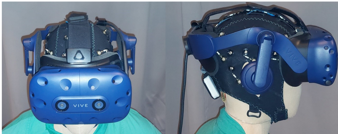
FIGURE 3 Experimental set-up for VR-testing: VR-headset combined with EasyCap recording cap and mobile EEG-device.
