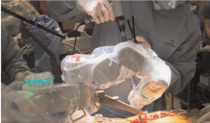
FIGURE 3 | Mazor X in working position during drilling of the pedicle for pedicle screw application.
