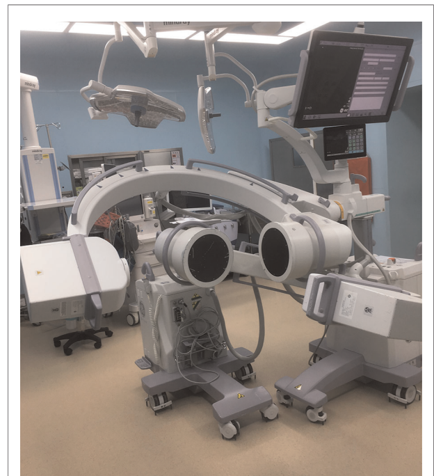
FIGURE 1 Two fluoroscopes were positioned with their image intensifiers kept perpendicular to each other.
