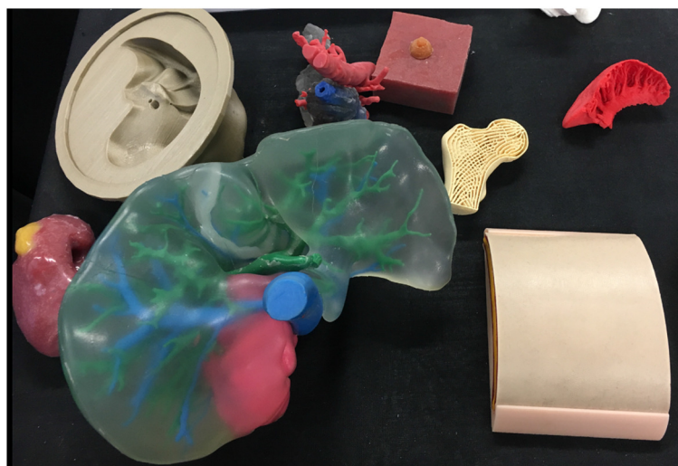
FIGURE 1 | A selection of models made via 3D printing or 3D printed molds including a renal tumor model (left), liver (center), femoral head (right), and skin (right).
