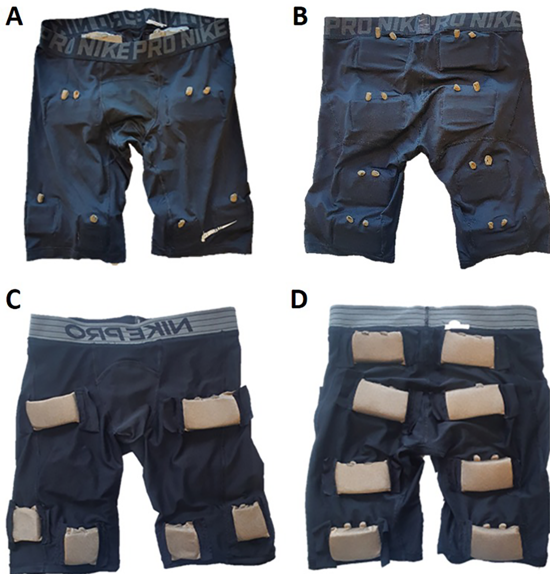
FIGURE 2 Image of NMES pants seen from the outside (A frontside, B backside) and inside (C frontside, D backside). On (A,B) there are connectors for stimulation. The larger electrodes are sized 5 × 9 cm (upper electrodes in C and all electrodes in D) and the smaller (lower electrodes in C) are sized 5 × 5 cm. The NMES pants are developed together with the Swedish School of Textiles at the University of Borås, Sweden. Image adapted from (12).
