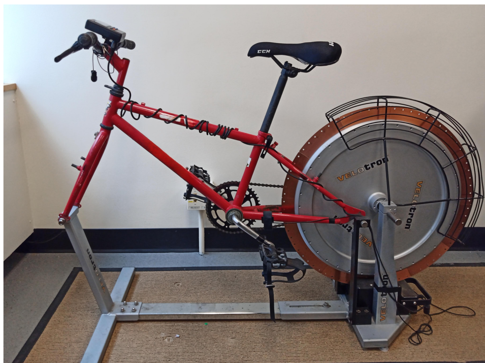
FIGURE 2 Electronic bike used for 30-s Wingate cycle ergometer test as modified for youth participants.
