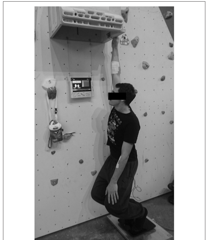
FIGURE 1 | Test setup. Participant standing on Entralpi© force plate, tablet for visual control at head height, one-hand pull on 23-mm rung.
