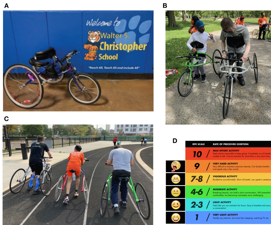
FIGURE 1 | (A) Running frame example. There are 3 wheels, a seat (styles of seat vary in shape and dimension), and a chest plate for additional trunk support. The front wheel is held steady with the use of a damper. Bicycle style breaks on the front wheel allow athletes to stop and wheel locks on one or both back wheels secure the frame for mounting and dismounting. The model shown here is by Petra (Peterson et al., 2015). (B) Front view of athletes using a running frame during a social and emotional learning (SEL) teamwork activity at practice. Both frames are by RAD (Black, 2021). (C) Back view of running frames in use during an endurance portion of practice by three athletes on a track to show relative width of the back wheels; they are wide enough for stability and fit through ADA-compliant doorways. The frames on right and left are RAD (Black, 2021), and middle is Eagle Sportschairs (Ewing, 2021). (D) Rate of perceived exertion (RPE) scale image used by athletes to report their perceived level of effort. This image was shown on shared screen during virtual sessions, and on a laminated index card during in-person sessions.
