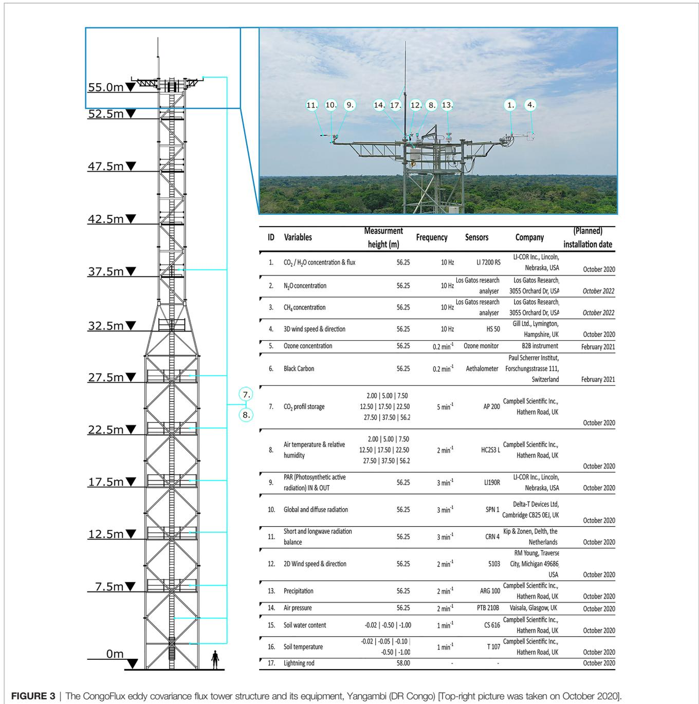
**FIGURE 3** | The CongoFlux eddy covariance flux tower structure and its equipment, Yangambi (DR Congo) [Top-right picture was taken on October 2020].
