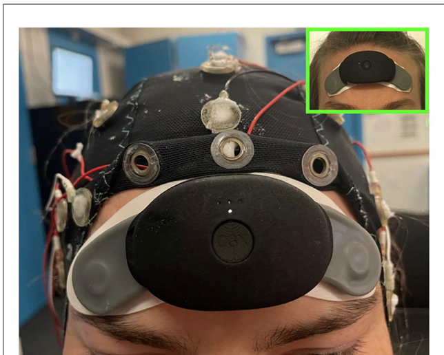
FIGURE 1 Picture of a subject wearing the CGX patch and EEG cap concurrently in order to collect both forehead EEG for spectral scoring and cap data for visual scoring. In the upper right is a picture of the CGX patch worn alone to show its minimal footprint as a sleep tracking device.
