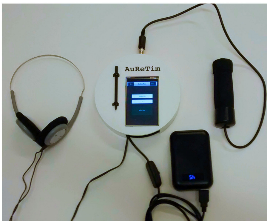
FIGURE 1 Photograph of the AuReTim psychomotor vigilance test with the device itself with the touchscreen and an attached touchscreen pen in the center, headphones at the left, hand-held push button at the right, and the switchable battery pack for portable usage at the lower right of the device.
