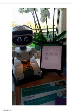
Setup of the Guardian system with the Misty robot.
