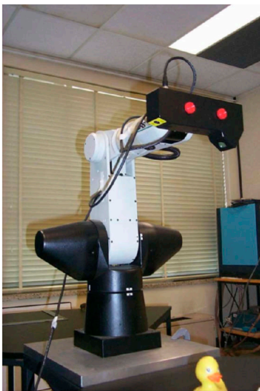
FIGURE 8 Biris range scanner on the end-effector of a CRS A465 6-DOF articulated manipulator. (Greenspan and Yurick, 2003).
