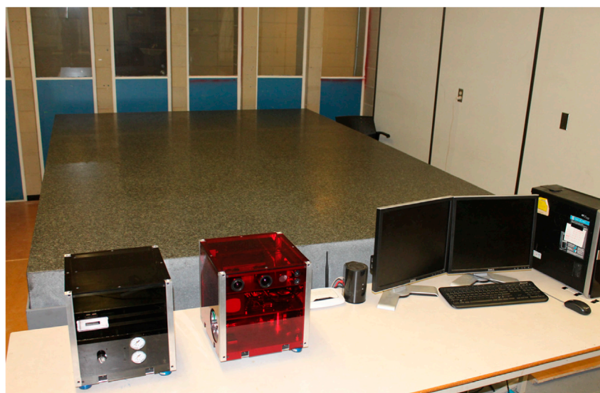
FIGURE 18 Spacecraft proximity operation testbed at Carleton University. (Ulrich and Hovell, 2017).
