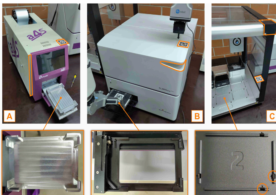
FIGURE 11 Photographs that show the three real instruments used to test the “CV + TF” method. (A): Plate sealer, (B): Plate reader, (C): Pipetting station. The important implementation details are highlighted in orange, while the photographs in the second row show the instruments’ handover position.
