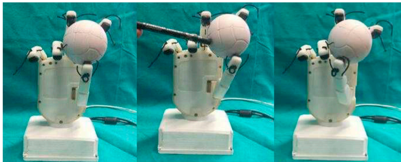
FIGURE 22 Frames during application of external disturbance.
