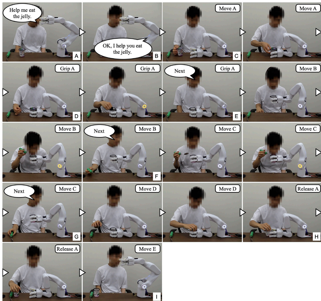
FIGURE 9 The work support of the “eating a jelly cup” task based on the learned data. (A) Participant inputs task name; (B) Work support for target task is initiated; (C) Move A is performed automatically; (D) Grip A is performed when cup is brought into system’s hand; (E–G) Move B, Move C, and Move D are triggered by voice command “Next”; (H) Release A is performed as participant attempts to receive cup with unaffected arm; (I) Move E is performed automatically.
