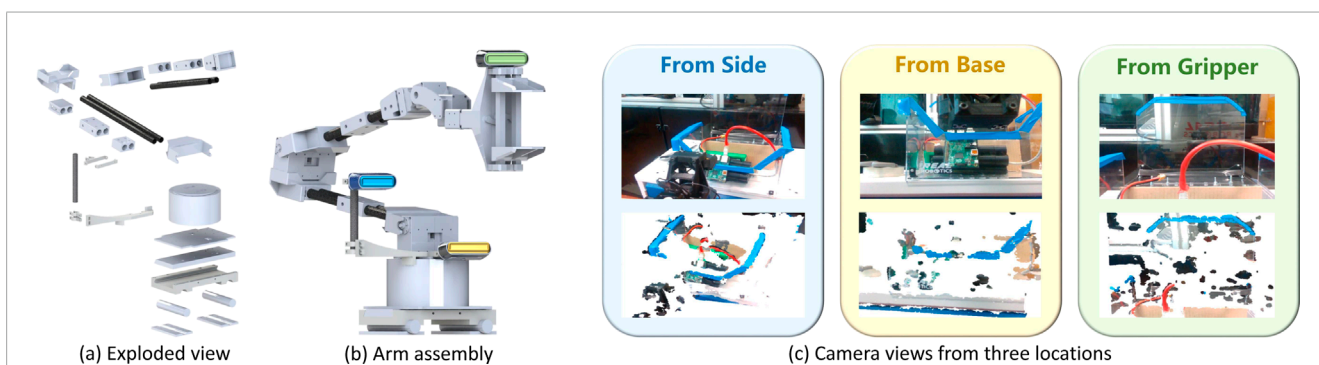
FIGURE 3 (A) Exploded view of all redesigned components in the robotic arm, (B) full assembly of the robotic arm with three possible camera mounting positions colored and (C) the corresponding RGB and depth camera image from each mounting location on the robotic arm.
