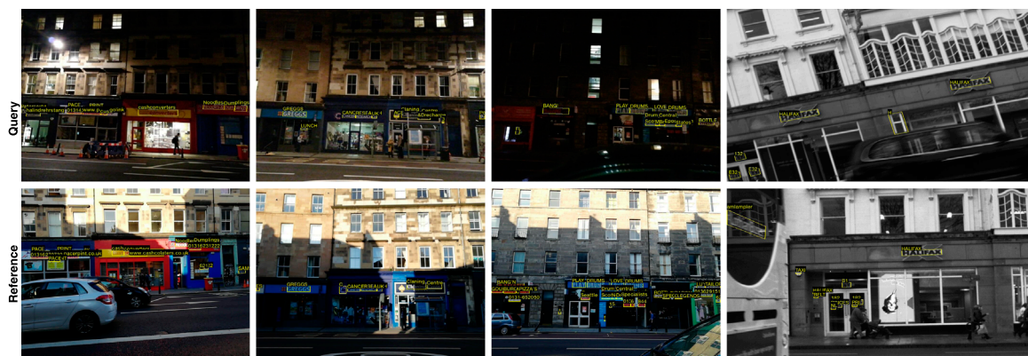
FIGURE 3 Sample query (top column)-reference (bottom column) frame pairs with text spotting results using the SCTP dataset (Hong et al., 2019). The proposed model spotted the majority of challenging cases of text instances in these frames. Best viewed when zoomed.
