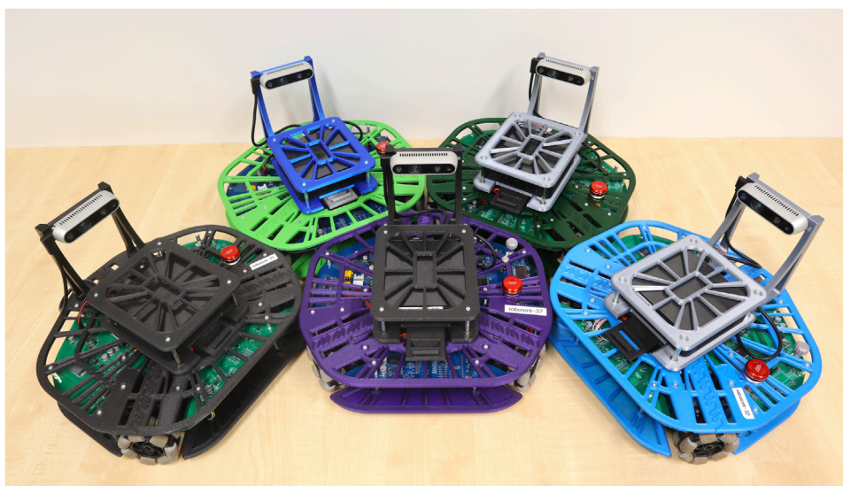
FIGURE 12 Different-coloured Robotont robots. The use of 3D-printing makes it possible to easily create different-coloured robots either for aesthetic or functional purposes.
