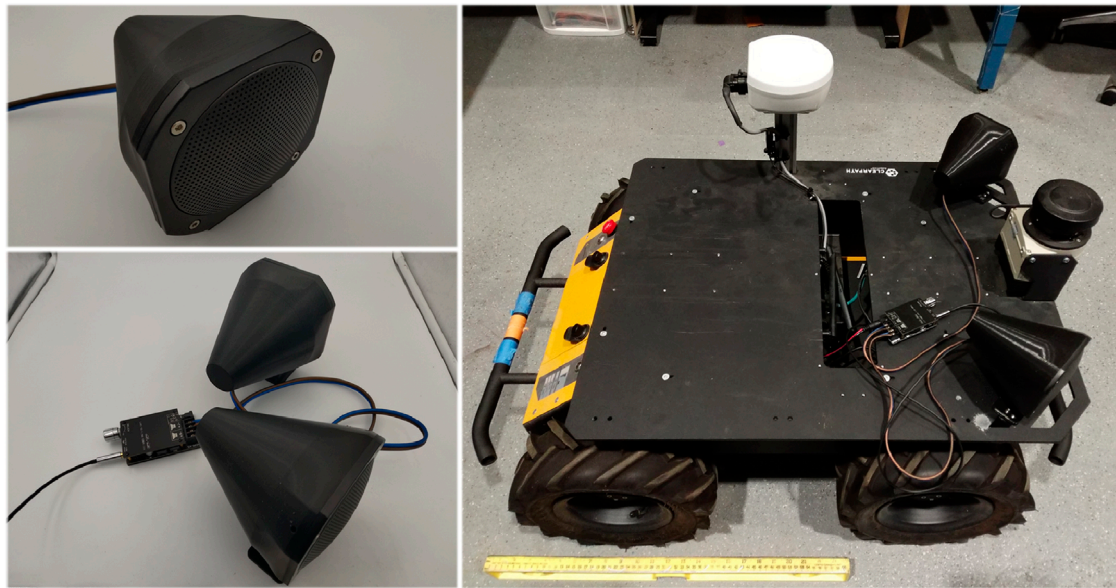
FIGURE 9 Top Left: the fully assembled speaker enclosure. Bottom Left: two-speaker system with the FRS 10 WP speaker driver and the TPA3116D2 amplifier module pictured fully connected. Right: Husky Robot with full system assembled.
