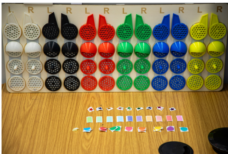
FIGURE 2 Physical customisation options provided to participants, showing 3D-printed parts for the robot's head and stickers for its body.
