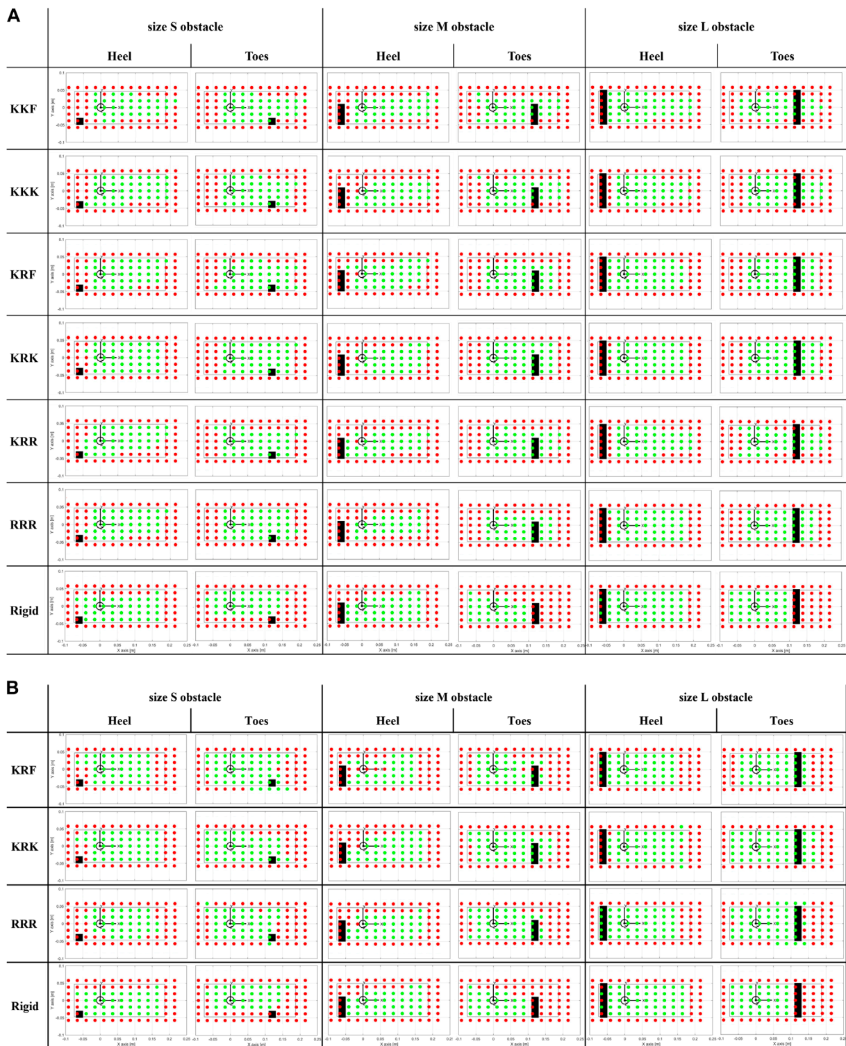
FIGURE 10 Stable (green dots) and unstable (red dots) points for different foot-obstacle combinations. The black inner rectangular profile represents the area of the unloaded tested foot (with the heel placed by the negative values of the x -axis); the origin of the reference frame coincides with the ankle projection; the black filled rectangle delineates the area of the obstacles. (A) The tested feet are the six SoftFoot configurations, and the rigid foot. (B) The tested feet are the three SoftFoot configurations with stiffer springs (springs constant 1.7 N/mm), and the rigid foot.
