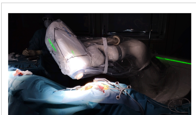
FIGURE 7 Operating room set-up during laser ablation. Robotic-assisted frameless laser osteotome in action.
