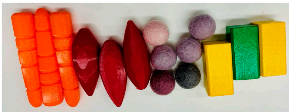
FIGURE 7 Objects used to evaluate single and multi-object grasping. From left to right: baby carrots, shallots, textile spheres representing cherry tomatoes, and wooden cuboids representing packaged goods.
