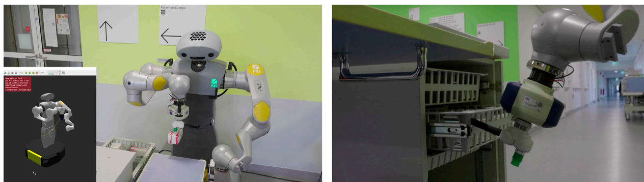
FIGURE 10 HoLLiE fetching a medicine box from a drawer and putting it on the table. Small picture shows the planned motion in the ArtiMinds RPS. This also required pulling out a drawer from a medicine cabinet. Picture taken at the demonstration days in the Hospital Karlsruhe.
