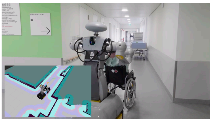
FIGURE 3 HoLLiE pushing a wheelchair around a curve in the Städtisches Klinikum Karlsruhe. The planned path is displayed on the real occupancy grid map of the hospital station.
