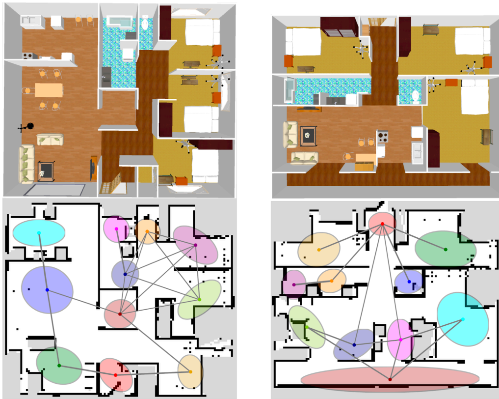
FIGURE 3 Overhead view of the simulator environments (top) and ideal spatial concepts expressed by SpCoTMHP on the environmental map (bottom) in Experiment I. The colors of the position distributions were randomly set. If (\psi_{k_1, k_2} + \psi_{k_2, k_1})/2 > 1/K , the centers \mu_{k_1}, \mu_{k_2} of the Gaussian distributions are connected by an edge. This means that the edges are drawn only if the average transition probabilities from k_1 to k_2 and k_2 to k_1 are higher than the uniform transition probability.
