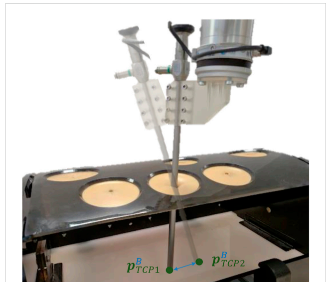
FIGURE 10 Linear movement performed to test the ff pivoting control for the Cartesian movement of the TCP.
