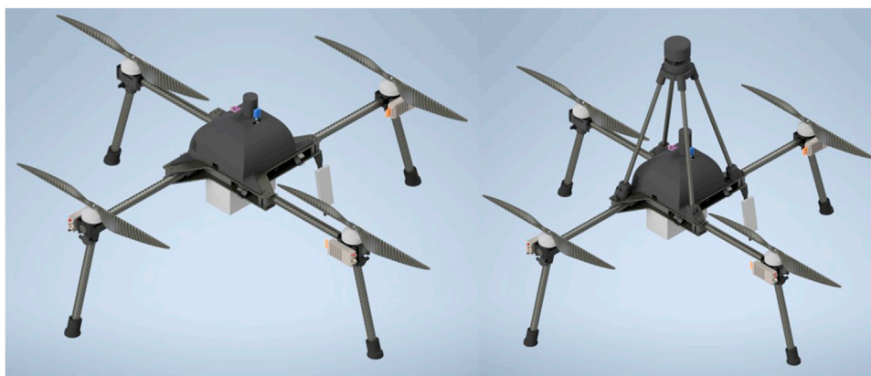
FIGURE Renders of the BUDS system with and without a sonic anemometer mounted.
