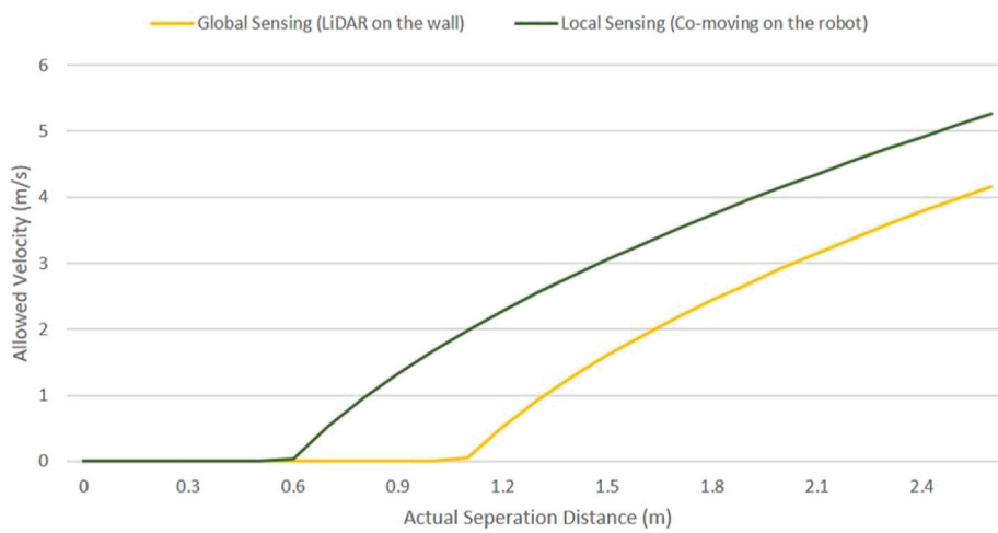
FIGURE 12 Safety distance and robot velocity for local (co-moving) and global collision sensing.
