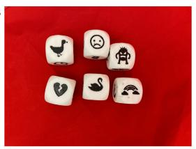
3D printed and laser engraved dice designed for this experiment.
