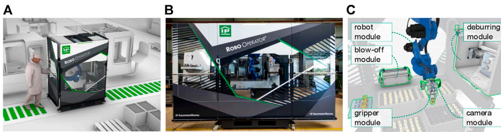
FIGURE 3 (A–C): The Robo Operator ® automates operator tasks on machine tools by skills.
