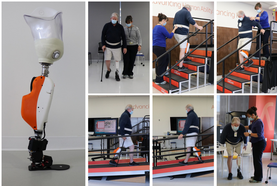
FIGURE 1 The powered knee and ankle prosthesis and participant training.
