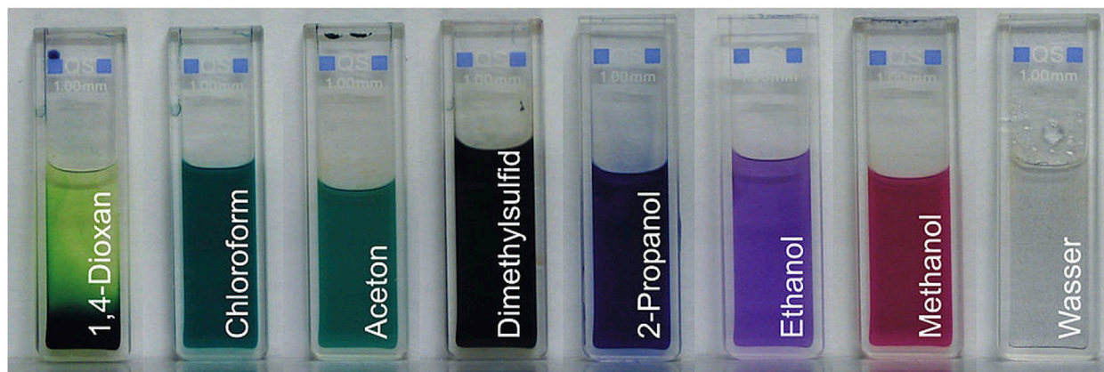
FIGURE 3 Reichardt's dye (Osterby and McKelvey, 1996) dissolved in different solutions (labeled). Dielectric constant, hydrogen bonding capacity and other properties of the solution affects the quantum excitations of the dye, changing its absorption and emission spectra.
