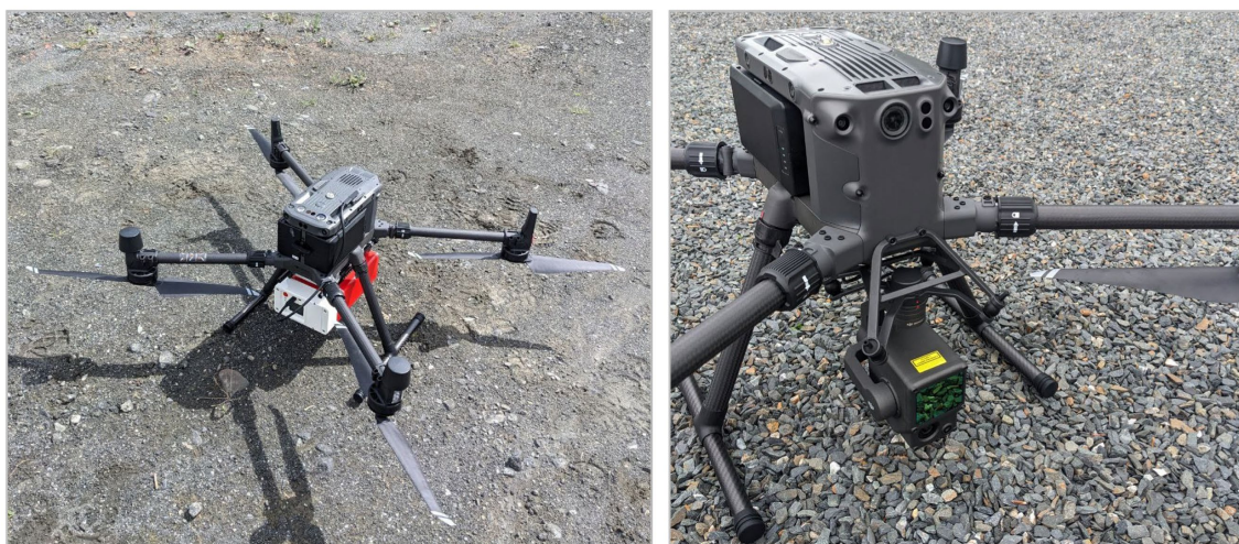
FIGURE 2 System for 3D radiation mapping including D230A gamma spectrometer (left) and Zenmuse L1 lidar sensor (right) mounted on a drone.
