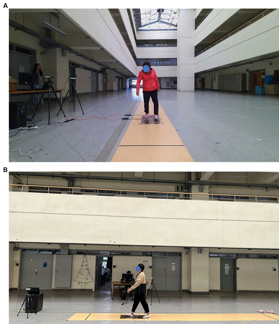
FIGURE 3 System setup for multimodal data collection system: (A) front view and (B) side view.
