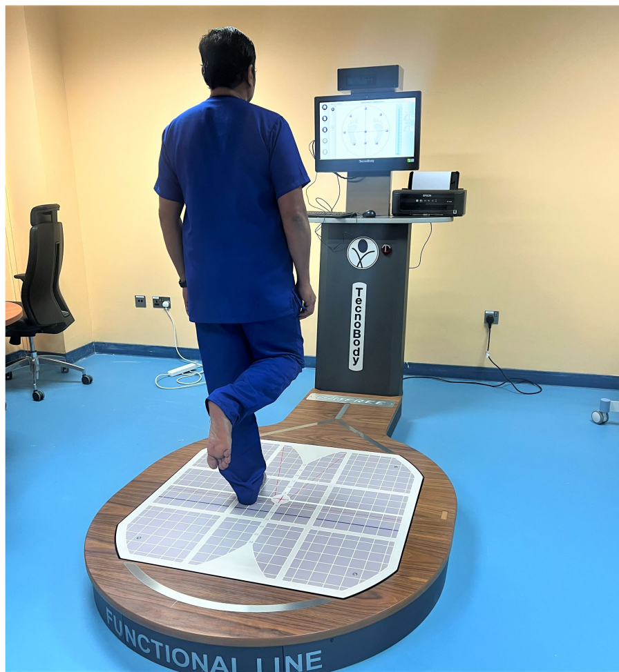
FIGURE 4 Computerized IsoFree stabilometric force platform for quantitative postural stability assessment in the study participants.
