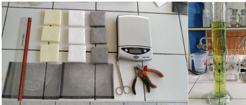
FIGURE 2 Tools for experimental determination of sorption capacity under atmospheric conditions.
