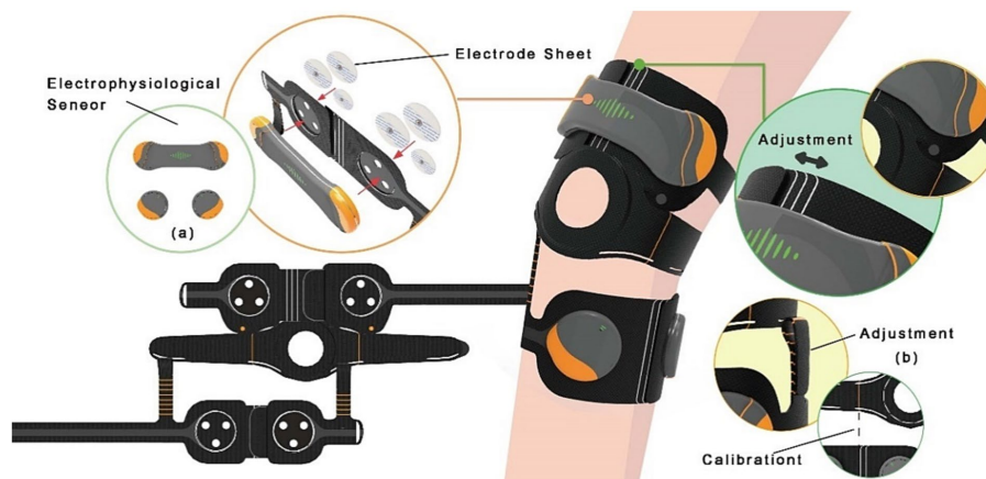
FIGURE 3 The design of the SSWAD with (A) the sensors and (B) detachable adjustment belt.
