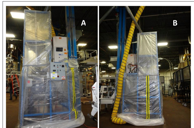
FIGURE 1 | Images of Grinder B (A) front view and (B) side view on 2nd and 3rd day of sampling with enclosure in place. One sampler was located inside the enclosure and the second sampler was located immediately outside the enclosure. The yellow and black stripes are the zippers to allow employee access and the yellow flexible tube is a ventilation duct.
