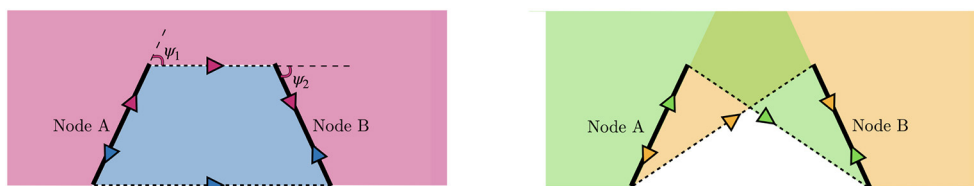
FIGURE 9 There are four possible permutations representing the interpolation between two edges in the image. Solid line denotes a node in a graph with the direction of travel indicated by the arrow. Dashed lines denote the interpolations. The two angles of interpolation, \psi_1 and \psi_2 are marked. Turning angle is the sum of the absolute values of these angles.
