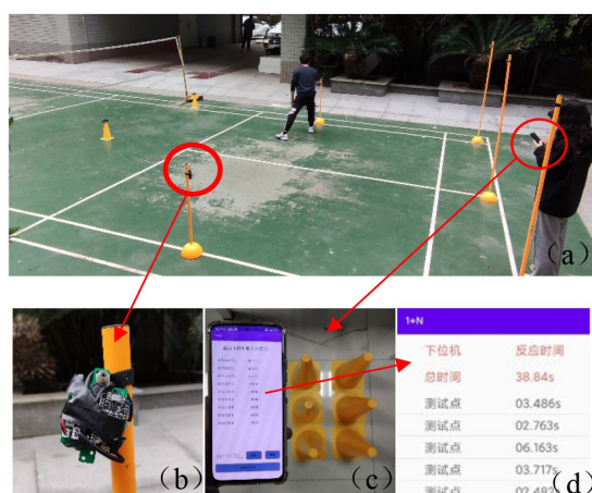
FIGURE 4 Agile training equipment. (a) training process, (b) lower computer, (c) upper computer application, (d) display interface.
