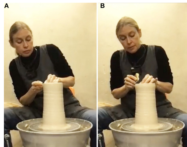
FIGURE 4 (A) The finished cylinder; (B) cutting off the top rim with a tool.
