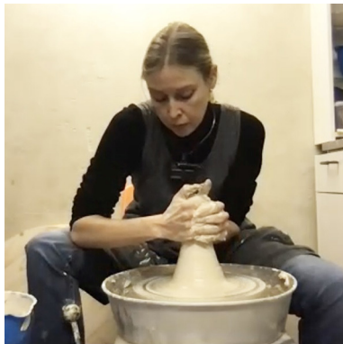
FIGURE 2 Centering the clay on the throwing wheel (repeated pushing up, pressing down).
