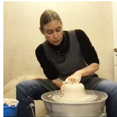
FIGURE 3 Making a hole and starting to prepare the base of the cylinder.
