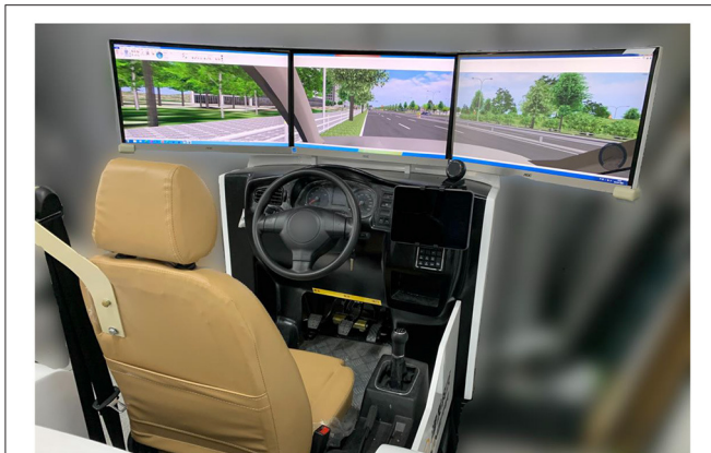
FIGURE 2 | The driving simulator used in the experiment: the condition of a physical present agent with low-level anthropomorphism.
