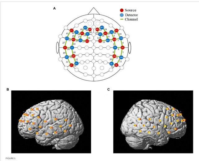
The locations of optodes and channels. (A) The locations of optodes and channels with respect to the EEG 10/20 system. The locations of sources (red dots) and detectors (blue dots) and 44 channels (green lines). (B) The locations of optical sources and detectors on a standardized 3D head on left view. (C) The locations of optical sources and detectors on a standardized 3D head on left view.
