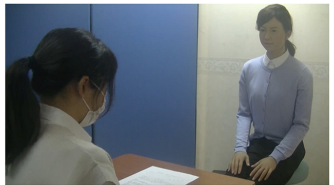
FIGURE 2 | An example of how an android robot provides exemplification. The researcher operated the android robot from a different room. When the researcher pushed a button, the robot began to speak exemplification according to previously prepared scripts. Participants then filled out their private narratives on the testing paper of SCT. Right: android robot; Left: participant.
