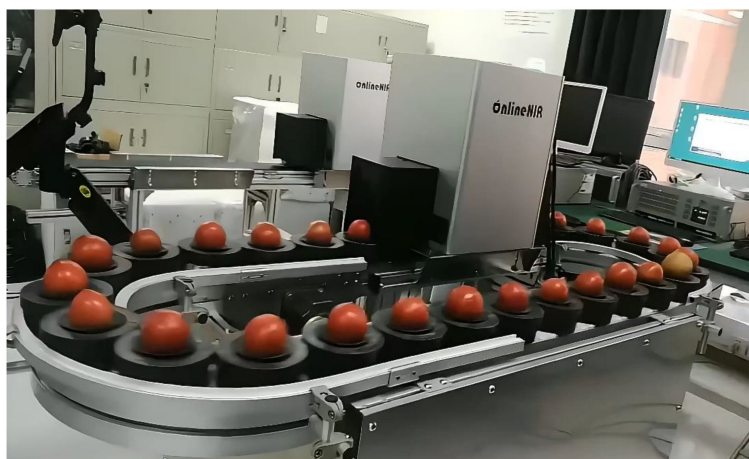
FIGURE 1 Full transmission Vis-NIR online tomato detection system.
