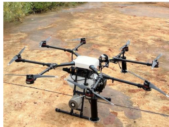
FIGURE 1 UAV and spraying system used in the test.
