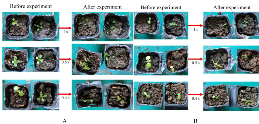
FIGURE 13 Diagram of the results of a laser weed control experiment. (A) 200 W NIR laser weeding experiment, (B) 100 W NIR laser weeding experiment.
